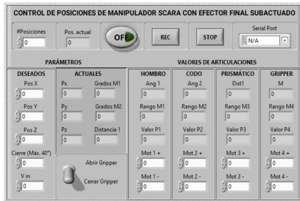
Fig. 4. Front panel to control and display the SCARA manipulator parameters.
